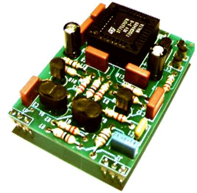
**PLM-24** is a low cost and easy to build Power Line Modem capable to send and receive serial data over the power lines (mains) at speed up to 2400 bps. **PLM-24** lets you communicate with other devices around the house without running any wires since it uses the wires already available in every house!
